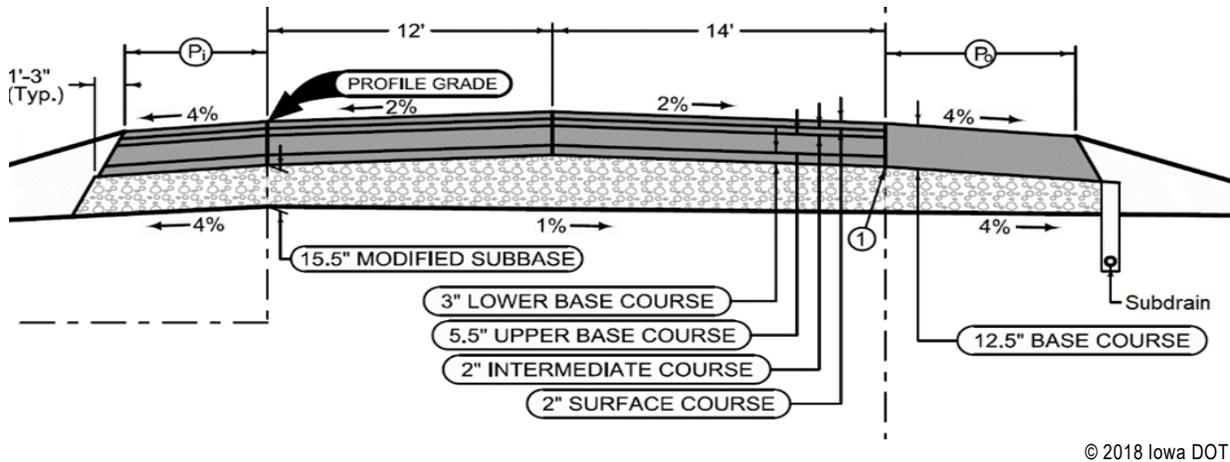
Figure 2. Iowa 100 pavement cross section design.
