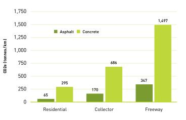
It should be noted that all the calculations in this paper are based on using 100 percent virgin materials for both the asphalt and concrete pavement options. In addition, only hot-mix asphalt pavements were analyzed consistent with the VicRoads project. If recycling and warm-mix asphalt were considered, the carbon footprint of the asphalt pavement would be further reduced.
