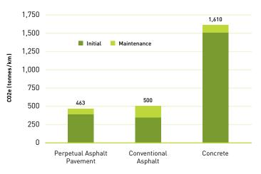
schedule used in the Ontario Life Cycle Cost Analysis model was analyzed. The details of the model are available in the paper. In addition, the life-cycle greenhouse gas emissions for all three options are shown in Figure 2.
