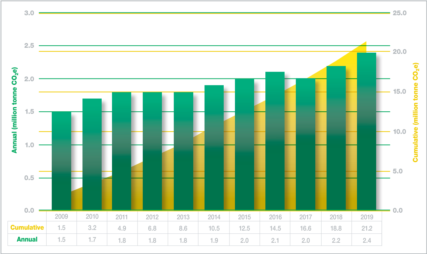
Figure 1. GHG Emissions Reduction from Use of RAP in New Asphalt Mixtures, 2009-2019
