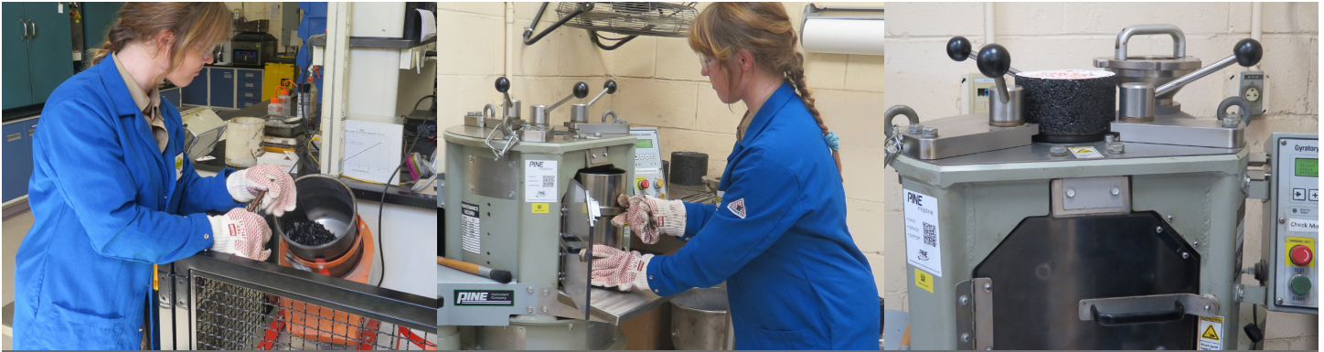
Colas HMA Lab Engineer Samantha Dixon mixes, compacts, and extrudes a test specimen in the lab. (credit: Colas Solutions Inc.)
