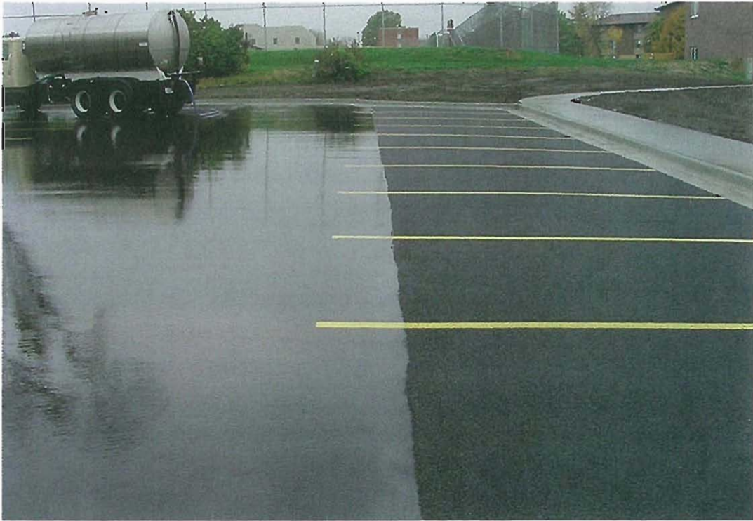
In a seniors' community in Iowa, a water truck demonstrates how porous pavement at the right drains quickly, while water stands on the conventional pavement at the left.
